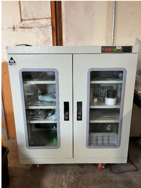
Electronic drying cabinet repurposed as a seed desiccator.
