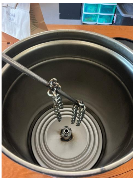
Inside the drum thresher: chains are welded in rows to the bottom of the drill bit.
